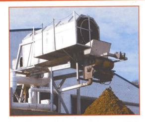
This Manure Separator is all stainless steel construction with self cleaning rotary screen, high flow capacities and excellent solid capture rates has low maintenance requirements, and handles any slurry content including sand.
